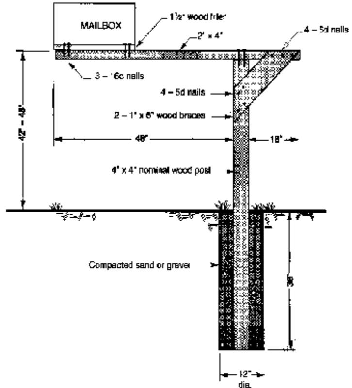
Figure 4: Example of a wood cantilever mailbox support.
